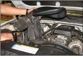
5. Disconnect the stock intake tube from the mass air sensor and from the throttle body, then, remove the intake tube as shown.
