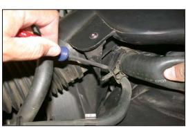
4. Unclip the radiator hose from the intake tube as shown.
