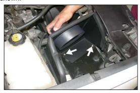
12. Install the heat shield onto the rubber mounted studs as shown.
