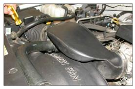
3. Loosen the hose clamps at the throttle body and at the mass air sensor.
