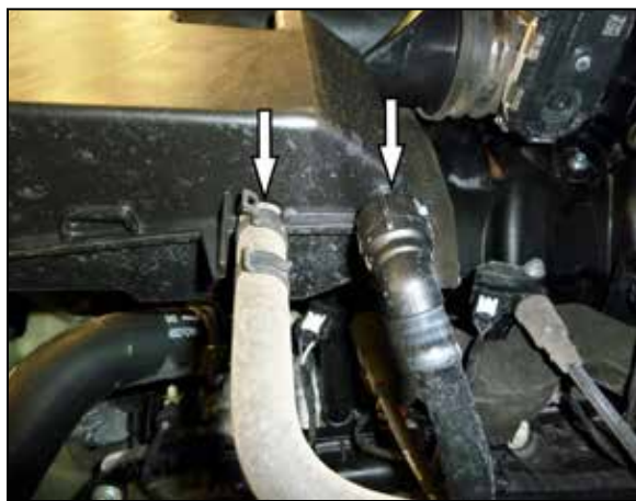
3. Disconnect the vent lines from the intake plenum.
