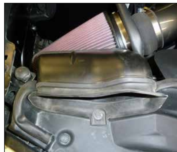
21. Reinstall the fresh air duct and secure with the factory push pin.
