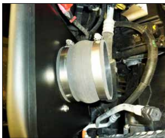
15. Install the provided hump coupler onto the filter adapter and secure with the provided hose clamp.
