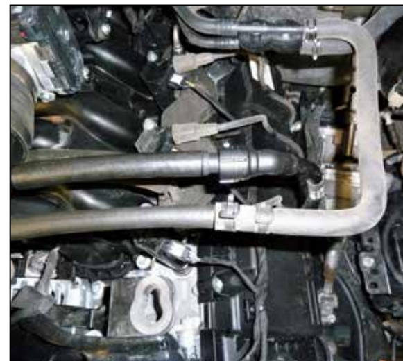
19. Connect the factory vent hoses to the hoses and fittings attached to the K&N intake tube.
