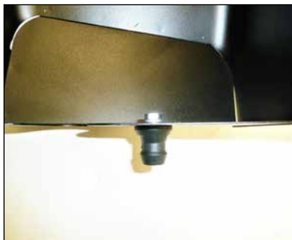
13. Install the mounting post onto the heat shield using the provided hardware.
