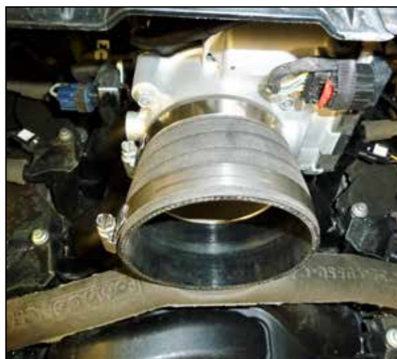
16. Install the straight coupler onto the throttle body and secure with the provided hose clamp.
