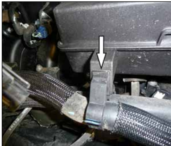
4. Unhook the vent line holder from the intake plenum.
