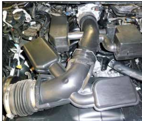
6. Lift the intake plenum up to dislodge it from the mounting grommets and then remove it from the vehicle.
