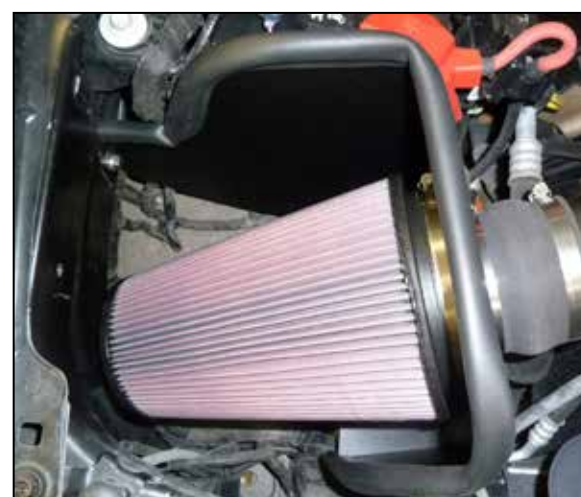
20. Install the K&N air filter onto the filter adapter and secure with the provided hose clamp.
