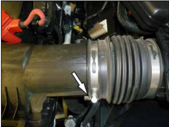
2. Loosen the hose clamp that secures the factory intake hose to the air filter housing.
