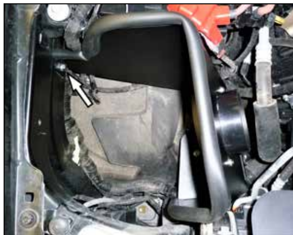
14. Install the heat shield so the mounting stud inserts into the mounting grommet and then secure to the inner fender with the provided hardware.
