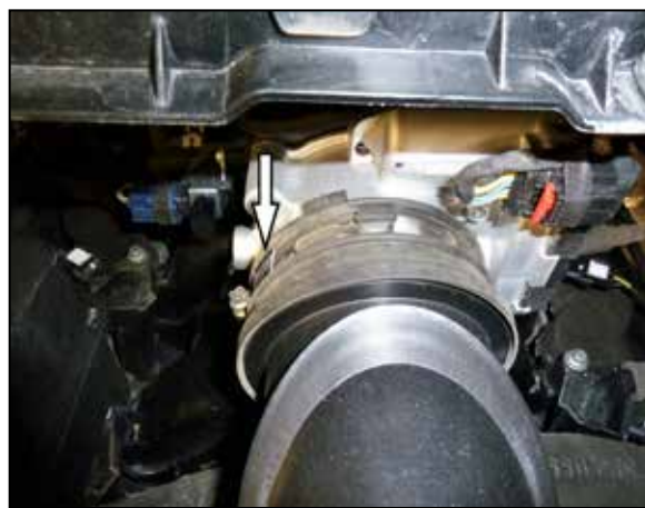
5. Loosen the hose clamp that secures the intake plenum to the throttle body.
