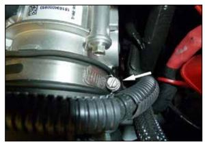
2. Loosen the hose clamp that secures the intake tube to the throttle body.
