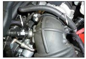
3. Disconnect the crank case vent hose from the factory intake tube and unhook the vent line that is attached to the tube.
