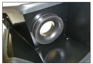
10. Install the provided filter adapter into the heat shield as shown using the provided hardware.
