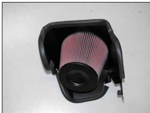
13. Install the K&N® air filter onto the filter adapter and secure with the provided hose clamp.
