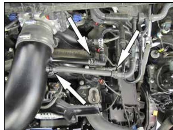
21. Install the shorter vent hose assembly onto the K&N® intake tube and then connect the other end into the EVAP vent line.
