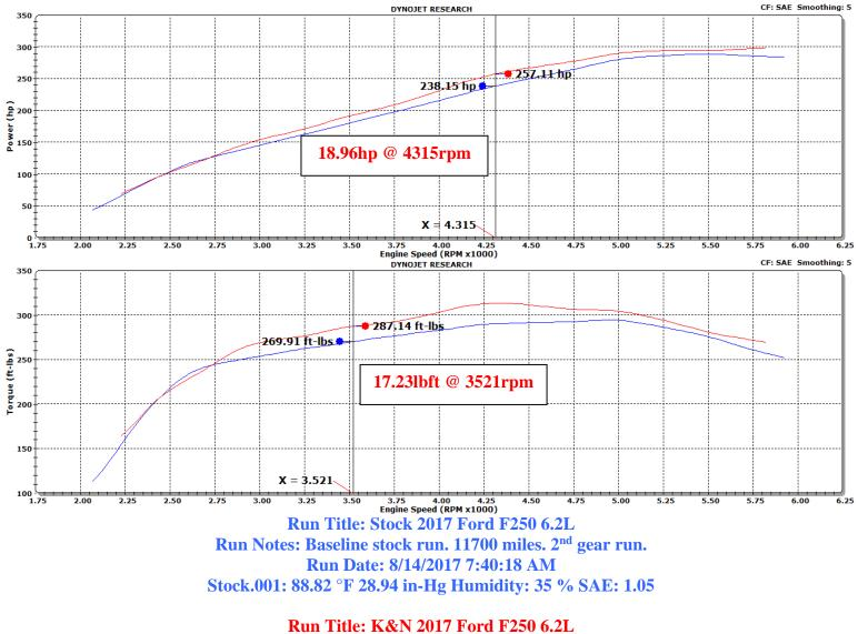
Run Title: K&N 2017 Ford F250 6.2L Run Notes: K&N intake kit #77-2588 installed. 11700 miles. 2<sup>nd</sup> gear run. Run Date: 8/14/2017 8:29:49 AM K&N.002: 96.38 °F 28.97 in-Hg Humidity: 27 % SAE: 1.05
