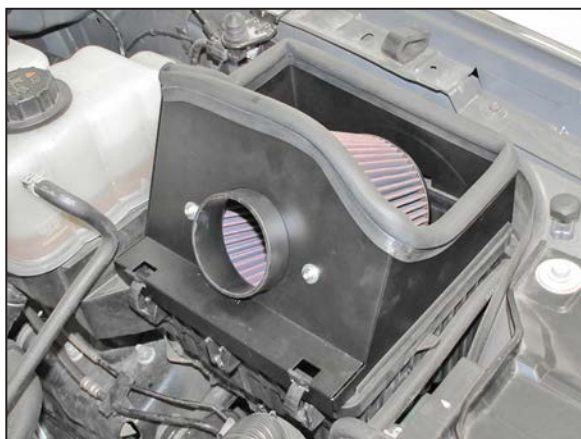
13. Install the heat shield/filter assembly onto the lower air box and secure with the two remaining factory clips.
