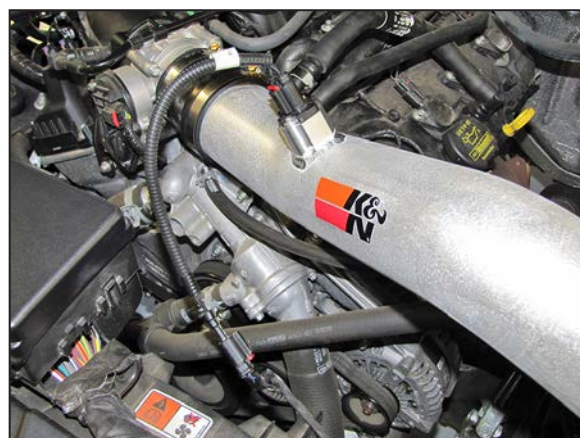
20. Connect the provided mass air extension harness into the factory wiring harness and then connect the other end onto the mass air sensor.
