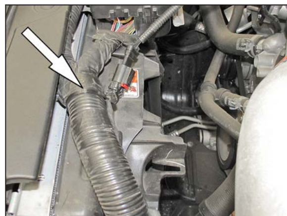
21. Secure the mass air wiring to the factory wiring harness with the provided tie wrap.
