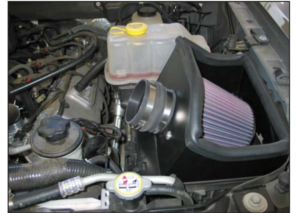
18. Install the provided silicone hump hose (08699) onto the filter adapter and secure with the provided hose clamps.
