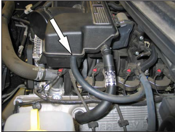
8. Disconnect the EVAP vent line from the intake plenum.
