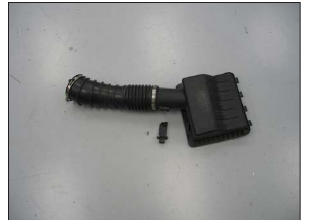
19. Remove the two screws securing the mass air sensor into the factory air box and then remove the mass air sensor from the air box.
