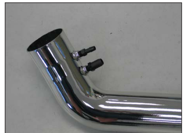
21. Install the two provided vent fittings into the K&N® intake tube as shown.
