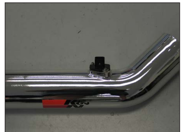
20. Install the mass air sensor into the K&N® intake tube as shown and secure with the provided hardware.
