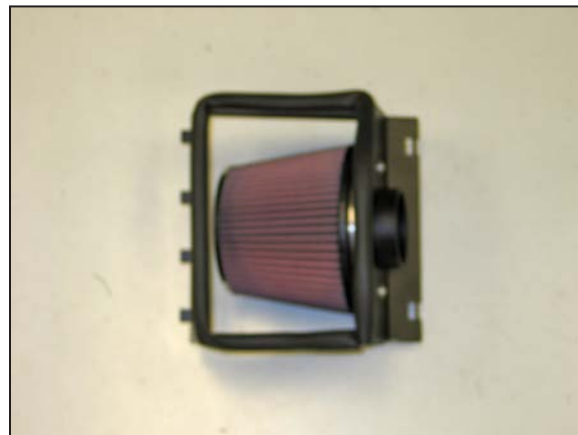
15. Install the K&N® air filter onto the filter adapter and secure with the provided hose clamp. NOTE: Drycharger® air filter wrap; part # RC-5173DK is available to purchase separately.
