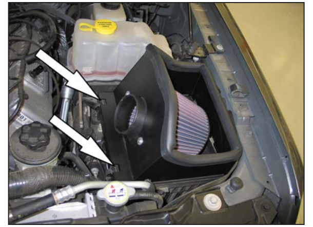
17. Set the heat shield assembly into the lower air box and secure with the two factory air box retaining clips.
