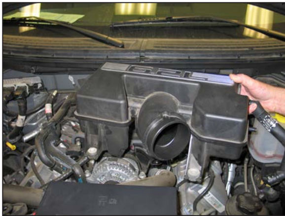
9. Loosen the hose clamp securing the intake plenum to the throttle body and then remove the intake plenum from the vehicle.
