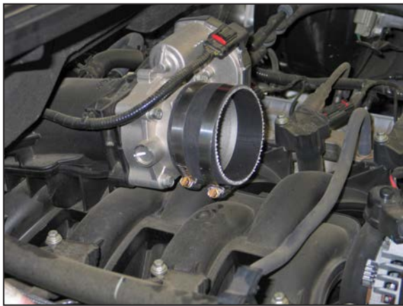
10. Install the provided silicone hose (08698) onto the throttle body and secure with the provided hose clamp.
