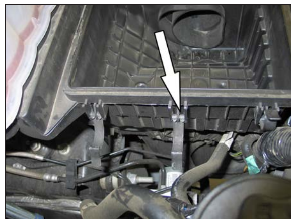
16. Remove the middle upper air box retaining clip from the lower air box.
