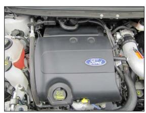
28. Reinstall the engine cover and secure with the factory hardware.
