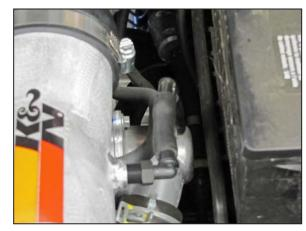
21. Using the provided 3/8" hose, connect the EVAP vent line to the 90° fitting installed into the K&N® intake tube.
