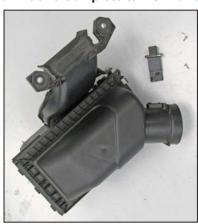
16. Remove the two screws securing the mass air sensor into the factory air box and then remove the mass air sensor from the air box.
