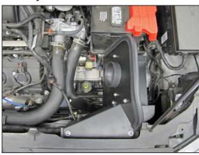
14. Install the heat shield assembly into the engine compartment so the heat shield stand-offs insert into the air box mounting grommets. Secure the fresh air intake scoop to the factory location using the provided hardware.
