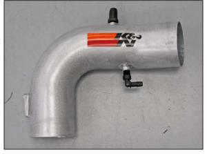
15. Install the 90° vent and the straight vent fitting into the  $K\&N^{\circ}$  intake tube as shown.
