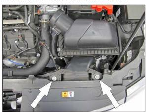
8. Remove the two bolts securing the fresh air intake scoop to the core support.
