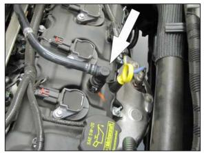
5. Rotate the locking tab and then disconnect the crank case vent tube from the valve cover.
