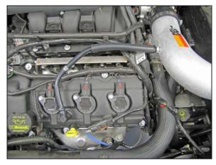
25. Reinstall the crank case vent tube onto the valve cover port and then install the open end to the fitting installed into the K&N® intake tube as shown.
