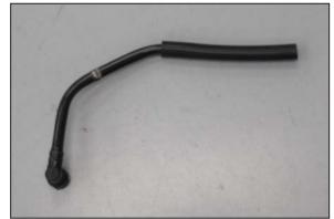
24. Install the provided 5/8" silicone hose onto the cut factory crank case vent tube as shown.
