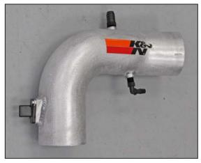
17. Install the mass air sensor into the K&N® intake tube and secure with the provide hardware.
