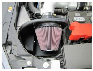
27. Install the  $K\&N^{\odot}$  air filter and secure with the provided hose clamp.
