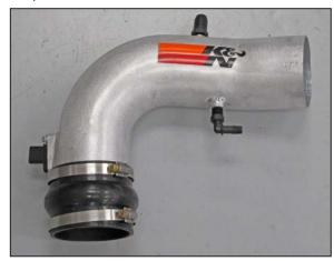
19. Install the silicone hump hose (084057) onto the K&N $^{\!\scriptscriptstyle \odot}$  intake tube as shown.
