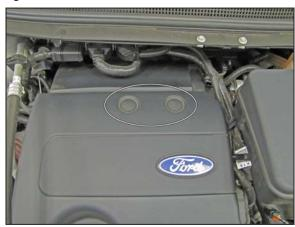
4. Remove the two push pins securing the rear of the engine cover and then remove the engine cover from the vehicle.
