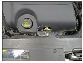
3. Remove the nut securing the front of the engine cover.
