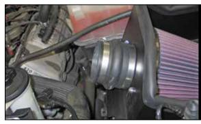
15. Install the provided silicone hump hose (5-576) onto the filter adapter and secure with the provided hose clamp.
