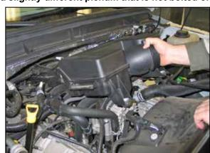
8. Unhook the heater hose clip from the intake plenum and then remove the plenum from the vehicle.
