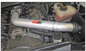
19. Install the K&N® intake tube into the silicone hose at the air filter and then into the silicone hose at the throttle body and secure with the provided hose clamps.
