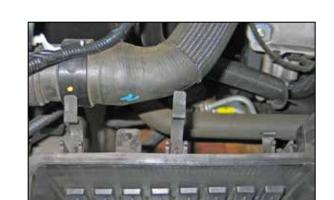
12. Remove the center upper air box retaining clip from the lower air box.
