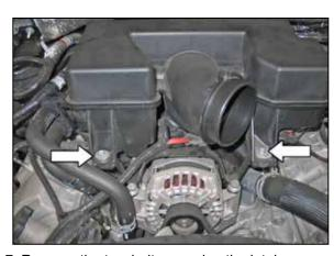
7. Remove the two bolts securing the intake plenum to the intake manifold and then loosen the hose clamp securing the plenum to the throttle body.
