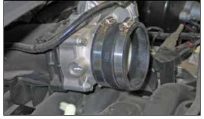
14. Install the provided silicone hose (08630) onto the throttle body and secure with the provided hose clamp.
