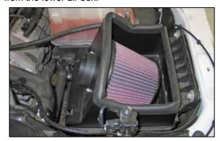
13. Install the K&N® filter/heat shield assembly and secure with the two remaining factory upper air box retaining clips.
