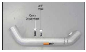
16. Install the quick disconnect and 3/8 NPT vent fittings into K&N® intake tube as shown.
