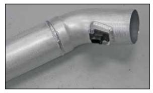
18. Install the mass air sensor into the K&N® intake tube and secure with the provided hardware.
