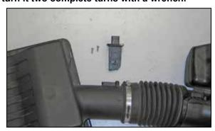
17. Remove the mass air sensor from the factory air box.
