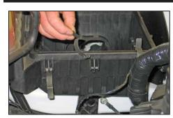
12. Remove the center airbox retaining clip.
