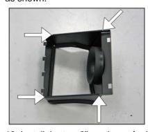
10. Install the two 9" sections of edge trim onto the bottom of the heat shield as shown.
