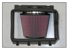
13. Install the  $K\&N^{\textcircled{8}}$  air filter onto the filter adapter and secure with the provided hose clamp.
