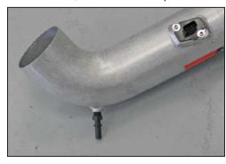
19. Install the provided crankcase vent fitting into the  $K\&N^{\circledR}$  intake tube as shown.
