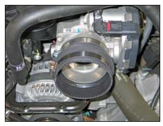
16. Install the provided silicone hose (08699) onto the throttle body and secure with the provided hose clamp.
