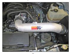
20. Install the K&N<sup>®</sup> intake tube; insert the lower end into the silicone hose attached to the heat shield /air filter assembly. Attach the upper end of the intake tube to the silicone hose secured to the throttle body. Secure the intake tube with the provided hose clamps.
