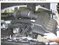
6. Remove the upper airbox housing and intake tube assembly from the vehicle.
