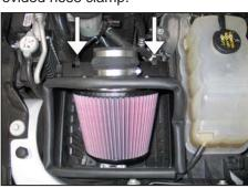
15. Install the completed heat shield/filter assembly onto the lower airbox. Secure with the two factory airbox retaining clips.
