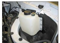
16. Secure the coolant bottle assembly to the inner fender using the provided hardware and spacer. NOTE: Only the front of the bracket will be mounted at this time. The spacer is to be placed between the inner fender and bracket.
