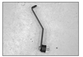
18. Install the provided rubber mounted stud onto the heat shield mounting bracket (083143) using the provided hardware.
