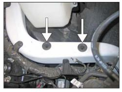
22. Remove the factory air box mounting grommets from the inner fender brace.
