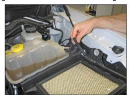
13. Lift the lower air box/coolant reservoir up to release it from the mounting grommets. Lean the coolant reservoir inward towards the engine, disconnect the coolant transfer hose from the coolant reservoir.
