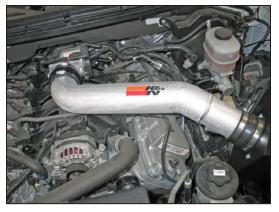
31. Install the K&N<sup>®</sup> intake tube into the silicone hose attached to the filter adapter. Insert the intake tube's opposite end into the silicone hose on the throttle body, secure each end with the provided hose clamps.
