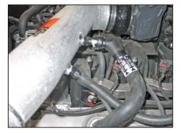
32. Connect the crankcase vent hose to the quick disconnect fitting. Attach the EVAP hose to the  $\frac{1}{2}$ " hose barb.
