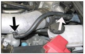
26. Attach the provided EVAP hose onto the fitting on the intake tube and then attach the open end to the EVAP check valve as shown.
