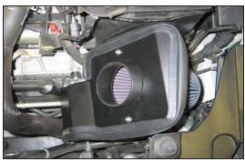
16. Set the heat shield onto the rubber mounted studs and then secure with the provided hardware. Install the K&N<sup>®</sup> air filter onto the adapter and secure with the provided hose clamp. **NOTE: Be sure to place the large fender** washers on top of the rubber mounted studs so that they are between the heat shield and rubber mounted studs.
