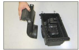
22. Remove the fresh air duct from the factory airbox.
