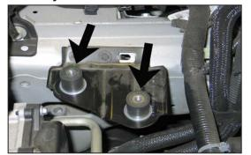
14.Install the provided rubber mounted studs onto
