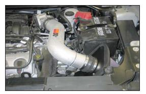
28. Reconnect the vehicle's negative battery cable. Double check to make sure everything is tight and properly positioned before starting the vehicle.
