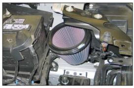
15. Set the K&N<sup>®</sup> air filter into the engine compartment as shown.
