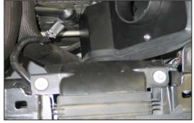
23. Install the fresh air duct into the heat shield and secure it with the factory screws in the original location, then reinstall the cover onto the core support.
