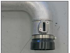
19. Install the remaining silicone hose (084073) onto the intake tube and secure with the provided hose clamp as shown.
