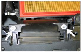
9. Remove the two bolts that secure the fresh air duct to the core support. NOTE: These bolts will be reused.
