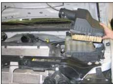
6. Remove the air box lid and stock air filter.
