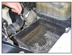
11. Remove the center air box lid mounting clip from the lower air box as shown.
