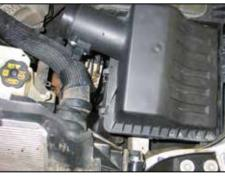
5. Release the three clips that secure the air box lid.
