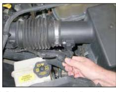
2. Release the red locking clip and then disconnect the mass air sensor electrical connection; unhook the wiring harness from the power steering reservoir.
