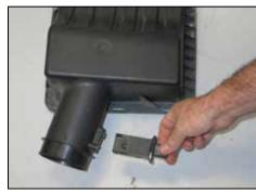
17. Remove the two screws securing the mass air sensor to the upper air box and then remove the mass air sensor from the upper air box.
