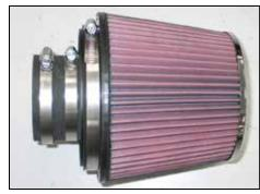
15. Install the silicone hose (08698) onto the filter adapter and secure with the provided hose clamp.
