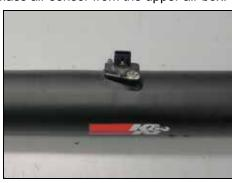
18. Install the mass air sensor into the K&N® intake tube and secure with the provided mounting screws.
