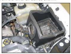
12. Install the heat shield assembly onto the lower air box and clip into place with the upper air box mounting clips.
