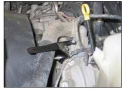
8. Install the tube mounting bracket (083111) and secure with the provided hardware and the bolt removed in the previous step.
