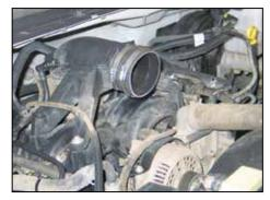
13. Install the provided silicone hose (08698) onto the intake plenum and secure with the provided hose clamp.
