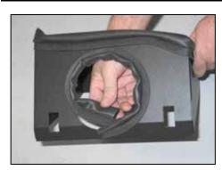
10.Install the provided edge trim into the hole in the heat shield as shown.
