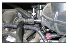
4. Rotate the locking tap and then disconnect the crankcase vent hose from the stock intake tube.
