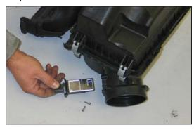
16. Remove the two screws securing the mass air sensor to the airbox and then remove the mass air sensor from the airbox.
