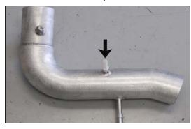
18. Install the provided 1/4npt fitting into the K&N® intake tube as shown.
