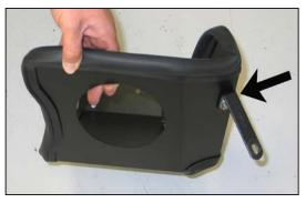
13. Install the provided "L" bracket (070094) onto the heat shield using the provided hardware as shown.
