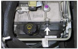
9. Remove the transmission pan bolt shown.
