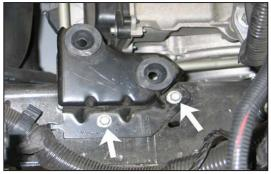
8. Remove the two bolts which secure the airbox mounting bracket to the inner fender.
