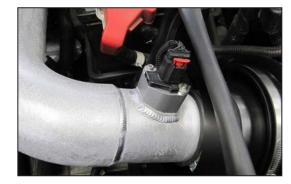
25. Using the provided mass air sensor extension harness, reconnect the mass air sensor electrical connection.
