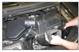
6. Remove the airbox from the vehicle.
