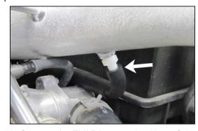
20. Connect the EVAP hose to the 1/4npt fitting as shown.
