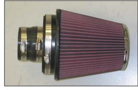
23. Install the silicone (084091) hose onto the filter adapter and secure with the provided hose clamp.
