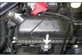
5. Loosen the hose clamp which secures the intake hose to the airbox. Remove the airbox mounting bolt shown.
