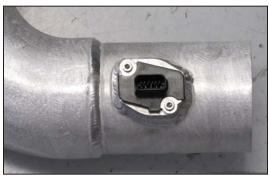
17. Install the mass air sensor into the  $K\&N^{\mbox{\scriptsize @}}$  intake tube and secure with the provided screws.
