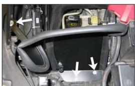
14. Install the heat shield into position on the inner fender and secure with the factory airbox mounting bracket bolts removed in step #8. Secure the heat shield mounting bracket to the airbox mounting bracket location on the core support using the factory bolt removed in step #5.
