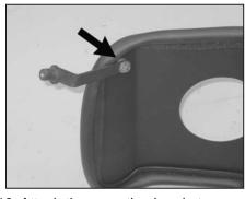
19. Attach the mounting bracket assembly to the heat shield with the provided hardware as shown. NOTE: Be sure to position the spacer between the bracket and heat shield.
