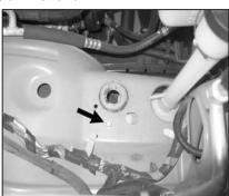
13. Remove the washer bottle mounting bolt shown.
