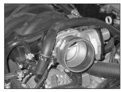
22. Install the silicone hose (08630) onto the throttle body and secure with the provided hose clamp.
