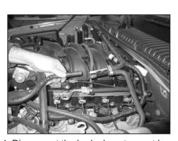
4. Disconnect the brake booster vent hose from the fitting as shown.
