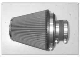
29. Install the silicone hose (08698) onto the air filter adapter and secure with the provided hose clamp.
