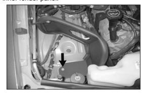
21. Secure the heat shield to the inner fender with the bolt removed in step #13 and the inserted nut and bolt.
