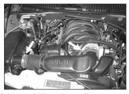
5. Loosen the hose clamps that secure stock intake tube to the throttle body and airbox shown.
