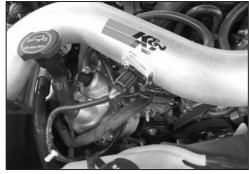
31. Reconnect the mass air sensor electrical connection.
