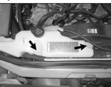
8. Loosen and remove the two bolts that secure the coolant recovery tank to the radiator.
