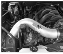
25. Install the K&N® intake tube into the silicone hose at the throttle body and align with the mounting bracket installed in step #22. Secure the intake tube with the hose clamp and supplied hardware.
