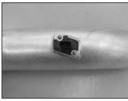
24. Install the mass air sensor assembly into the K&N® intake tube and secure with the provided hardware.
