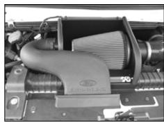
32. Install the factory fresh air scoop onto the heat shield and then latch it into the cut out and factory opening as shown.
