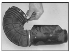
8a. On vehicles equipped with an external air temperature sensor; remove the air temperature sensor from the stock intake tube.
