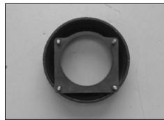
18. Install the mass air gasket to the filter adapter as shown.
