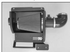
24. Install the  $K\&N^{\otimes}$  air filter onto the filter adapter and secure with the provided hose clamp.
