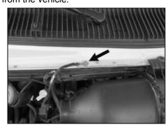
3. Remove the two bolts that secure the air filter assembly to the cowl.
