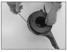
11. Use a screw driver to open the mass air sensor housing and remove the mass air sensor from the housing.
