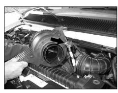
6. Lift up the air filter housing and unhook the mass air sensor secondary connector from the housing. Then disconnect the mass air sensor secondary connection and remove the filter assembly from the vehicle.
