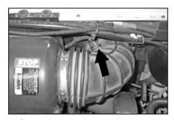
3a. On vehicles equipped with an external air temperature sensor; disconnect the temperature sensor electrical connection.
