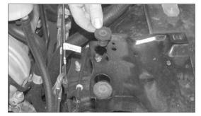
pull the crank case vent hose off of the valve cover.
