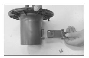
14. Remove the mass air sensor retaining screws and then remove the mass air sensors as shown.
