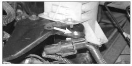
4. Unhook the secondary mass air sensor electrical connection from the power steering reservoir bracket, then unlock the electrical connection locking tabs and separate the electrical connection
