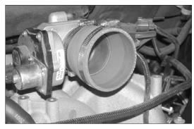
16. Install silicone hose (08724) onto the throttle body with the provided hose clamp as shown.
