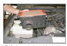
7. Pull firmly up on the lower air box housing to dislodge from the mounting grommets and remove lower air box from the vehicle.
