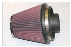
22. Install the provided adapter into the K&N $^{\! \otimes}$  air filter and secure with provided hose clamp as shown.
