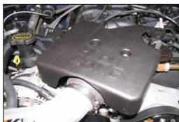
25. Reinstall the engine cover and secure with the factory mounting bolts.
