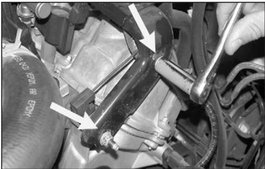
9. On vehicles equipped with the intake tube support bracket, remove the two nuts and then remove the stock intake tube support bracket as shown.
