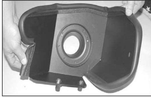
14. Install the provided trim seal onto the heat shield and trim to fit as shown.
