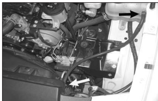
15b. Install the supplied coolant recovery hose and secure with the provided hose clamps. NOTE: Be sure to replace the coolant that was recovered during hose removal by replenishing it in the coolant recovery tank.
