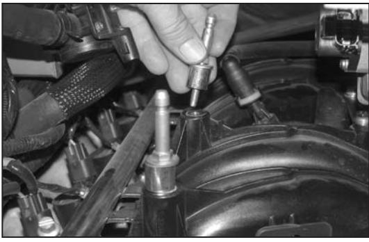
8a. Re-install the factory airbox mounting studs with the provided spacers as shown.
