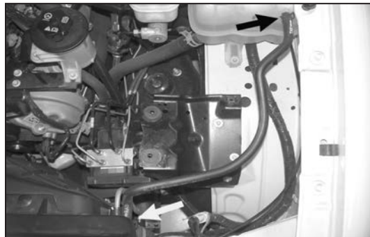
15a. Loosen the coolant recovery hose, hose clamps, and then remove the factory recovery hose shown. Be sure to catch any coolant, which flows out of the radiator during hose removal. NOTE: Be sure to let the engine cool completely before removing the overflow hose or hot coolant will escape from the radiator and injury or damage may result.
