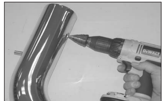
17b. Remove the intake tube and drill a 5/8" hole at the location marked in step #17a. NOTE: Be sure to remove all the burrs after drilling.
