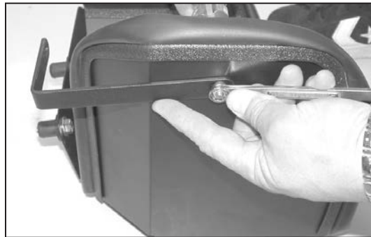
15. Install the provided "L" bracket onto the heat shield using the provided hardware as shown.
