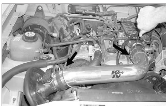
19. Slide the intake tube into the silicone hose at the throttle body and at the mass air sensor, adjust for best fit and tighten as shown.
