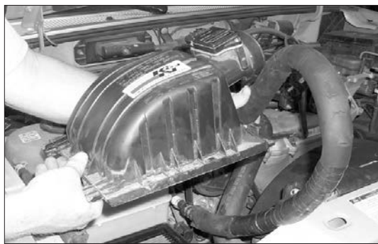
9. Unclip the air cleaner cover and remove as shown.
