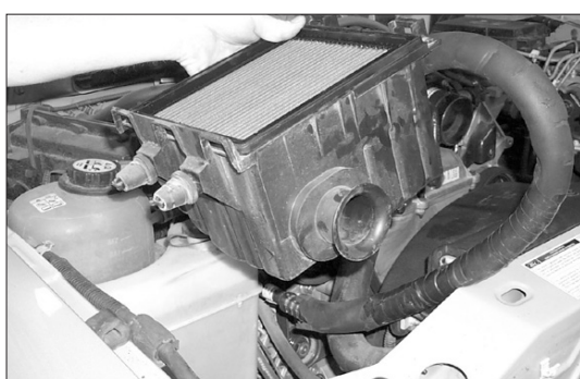
10. Using a flat blade screwdriver insert the blade between the air cleaner tray and the bottom of the lower air cleaner. Pry downward on the tray with the screwdriver while lifting upward on the air cleaner to release it from the stock grommets as shown. NOTE: K&N Engineering, Inc., recommends that customers do not discard factory air intake.
