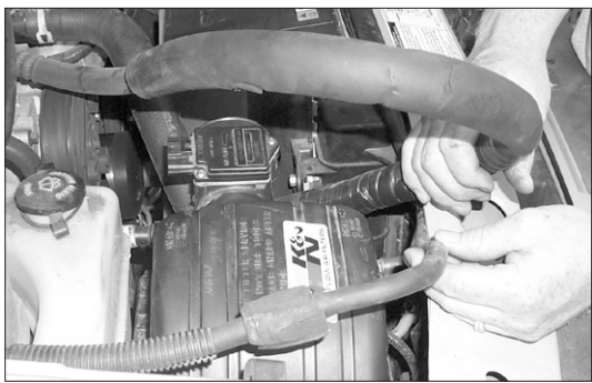
8. Rotate the air condition hard line and the coolant overflow line upward as shown.
