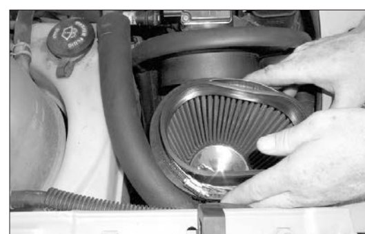
22. Squeeze the filter as shown and slide the filter into the inner fender as shown.
