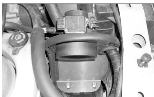
16. Install the heat shield assembly and line up the rubber expansion nuts into the holes on the air cleaner tray but do not tighten at this time.
