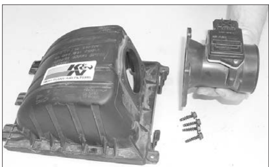
12. Remove the mass air sensor from the air cleaner cover as shown.
