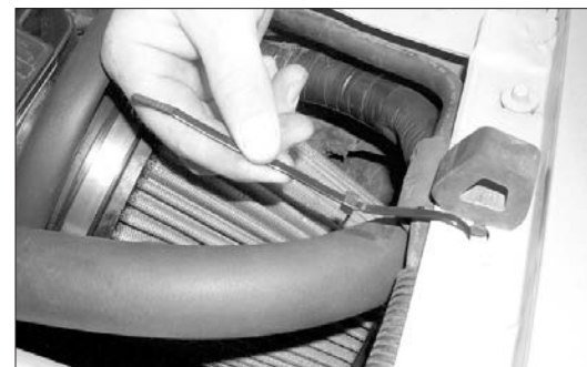
26. Using the provided zip-tie secure the air conditioning hard line and the coolant overflow hose to the inner fender as shown.
