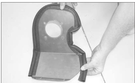
13. Install the provided edge trim onto the heat shield as shown.
