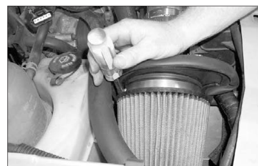
23. Slide the filter onto the mass air adapter and secure with the provided hose clamp as shown.
