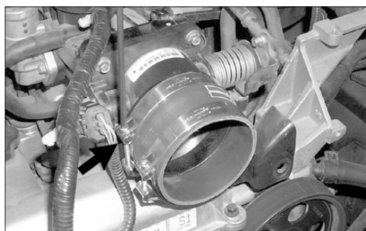
17. Install the silicone hose and hose clamps onto the throttle body and tighten as shown.
