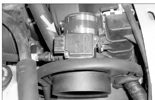
18. Install the silicone hose and hose clamps onto the mass air sensor and tighten as shown.
