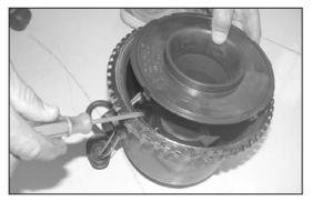
11. Using a flat blade screwdriver release the housing cover and pull up as shown.
