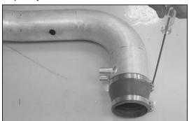
18. Install the provided silicone step hose and hose clamps onto the K&N® intake tube and tighten as shown.
