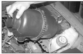
8. Pull firmly upwards to release the air cleaner assembly from the stock grommets located on the inner fender.
