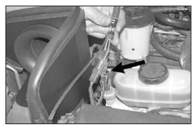
28. Reconnect the secondary mass air electrical connection as shown.
