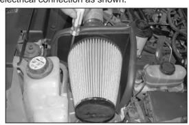
30. Install the  $K\&N^{\otimes}$  air filter and secure with the provided hose clamp as shown.
