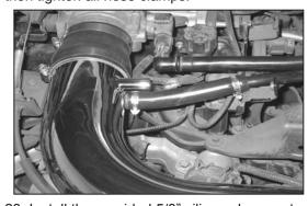
23. Install the provided 5/8" silicone hose onto the stock plastic crankcase vent line. Then, install the open end of the 5/8" ID silicone hose onto the  $K\&N^{\circledR}$  intake tube and secure with the provided hose clamps.
