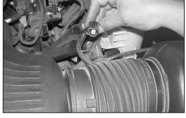
5. Disconnect the air temperature sensor electrical connection as shown.
