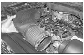
6. Loosen the hose clamps at the throttle body and at the air cleaner, then, remove the stock intake tube as shown.
