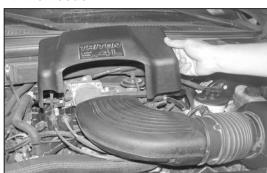
2. Remove the three engine cover bolts, then, remove the cover as shown.
