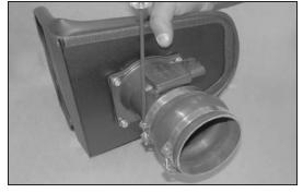
16. Install the silicone hump hose and hose clamps onto the mass air sensor and tighten as shown.
