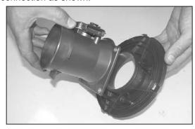
13. Remove the mass air sensor from the housing cover as shown.
