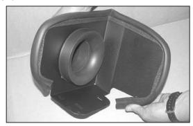
15. Install the provided edge trim onto the heat shield as shown.
