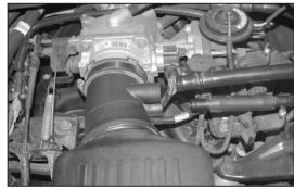
3. On vehicles with 5.4L engines, disconnect the crankcase vent hose and the idle air control vent hose from the stock intake tube as shown.
