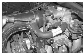
24. On vehicles equipped with a 4.6L engine, attach the provided 5/8"id idle air by-pass vent hose onto the appropriate fitting on the K&N® intake tube, trim for proper fitment to prevent the hose from developing a kink and attach the open end to the idle air by-pass valve.
