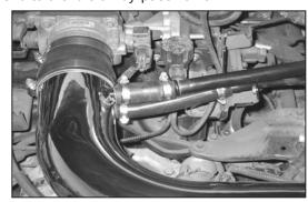
25. On V8-5.4L models slide the provided 5" long silicone hose onto the hard line, then trim hose for best fit before connecting to the vent on the  $K\&N^{\otimes}$  intake tube as shown.
