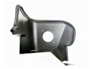
7. Install the provided edge trim onto the heat shield as shown. Some trimming of the edge trim will be necessary.
