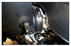
2. Disconnect the IAT sensor electrical connection and loosen the hose clamp that secures the intake plenum to the throttle body.
