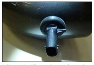
14. Remove the IAT sensor from the factory air filter housing and remove the O-ring from the sensor. Using the provided grommet, install the IAT sensor into the K&N intake tube. **NOTE: The IAT sensor is very fragile, be careful while handling the sensor.**
