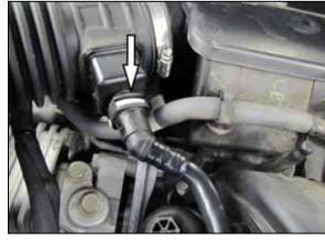
3. Release the locking tap and disconnect the crank case vent line from the factory intake tube.
