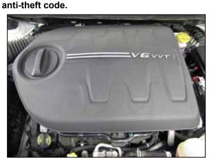
2. Lift off the engine cover and set aside.
