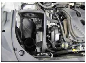
9. Install the heat shield into the vehicle so the mounting grommets and studs engage.
