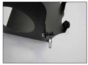
6. Install the air box mounting stud onto the K&N heat shield using the provided hardware.
