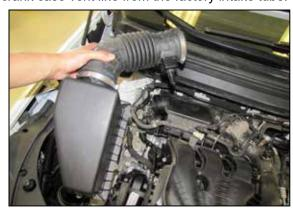
4. Loosen the hose clamp that secures the intake tube to the intake plenum. Disconnect the intake tube and then remove the complete intake system.
