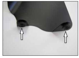
5. Remove the two factory mounting grommets from the factory air filter housing and install them into the K&N heat shield as shown.
