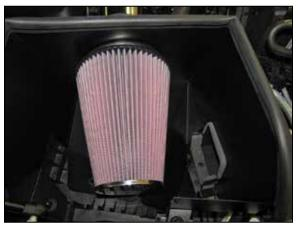
14. Install the K&N<sup>®</sup> air filter and secure with the provided hose clamp.
