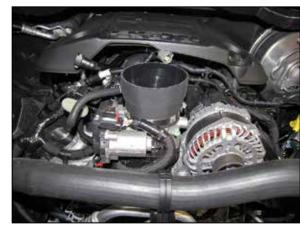
8. Install the provided coupler (08497) onto the throttle body and secure with the provided hose clamp.
