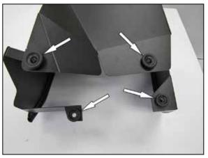
6. Remove the four mounting grommets from the factory air filter housing and install them into the heat shield as shown.
