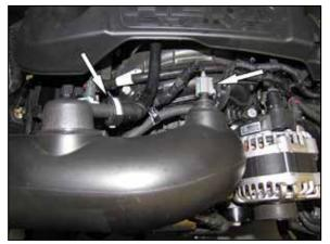
2. Disconnect the inlet air temperature sensor electrical connection and crank case vent line from the factory intake tube. 3. Loosen the hose clamp at the throttle body and then lift the complete intake system out of the vehicle.
