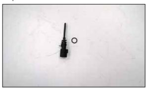
10. Remove the inlet air temperature sensor from the factory intake tube and remove the O-ring from the sensor.
