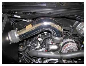
12. Install the K&N<sup>®</sup> intake tube into the coupler at the heat shield and then into the coupler on the throttle body, adjust the tube for best fit and then secure with the provided hose clamps.
