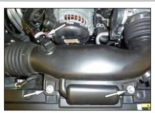
3. Remove the two bolts shown that secure the intake tube to the core support. Push the white
