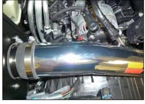
13. Connect the crank case vent line to the  $K\&N^{\otimes}$  intake tube.
