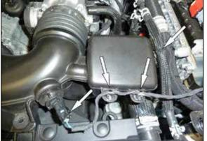
2. Disconnect the inlet air temperature sensor connection and unhook the wiring harness from the intake plenum. Unhook the coolant by-pass hose from the intake plenum and loosen the hose clamp that secures the tube to the throttle body. locking for the crank case vent line down and then disconnect the crank case vent line from the intake tube.
