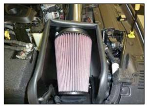
14. Install the K&N<sup>®</sup> air filter and secure with the provided hose clamp. NOTE: Drycharger<sup>®</sup> air filter wrap; part #
