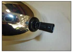
8. Install the provided grommet and factory temp sensor onto the K&N<sup>®</sup> intake tube.
