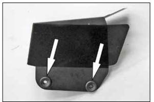
9. Install the two mounting grommets from the previous step into the K&N $^{\!@}$  heat shield as shown.
