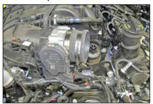
18. Install the provided step coupler onto the throttle body and secure with the provided hose clamp.
