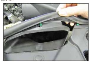
6. Unhook the hood seal mounting pin from the fresh air intake scoop.
