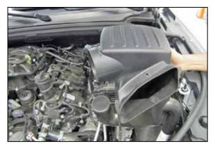
7. Lift up the air filter housing to dislodge it from the mounting grommets and then remove it from the
