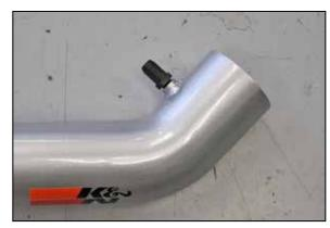
17. Install the provided vent fitting into the K&N® intake tube as shown.
