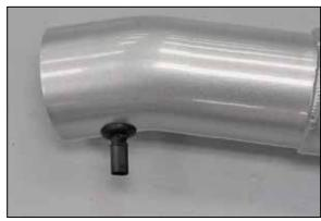
16. Install the provided grommet into the K&N® intake tube then remove the O-Ring from the inlet air temperature sensor and then install the sensor into the grommet install into the K&N® intake tube. NOTE: The inlet air temperature sensor is very fragile, use care while handling the sensor.
