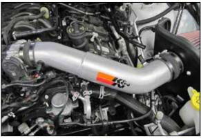
19. Install the K&N® intake tube into the coupler at the throttle body and then into the hump coupler, adjust the tube for best fit and then secure with the provided hose clamps.
