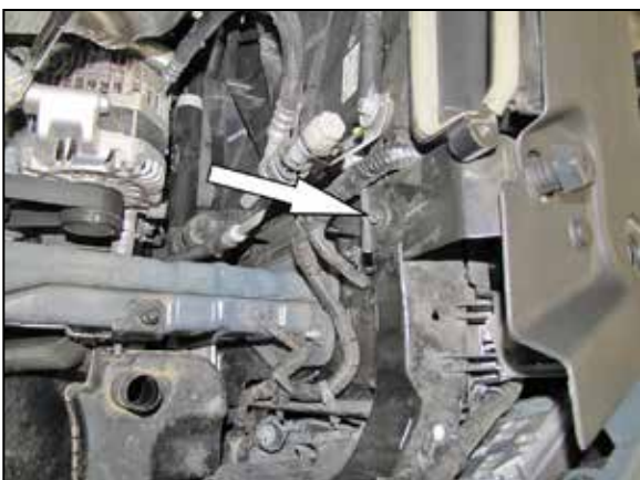
11. Remove the bolt shown from the core support. NOTE: This bolt will be reused in the next step.
