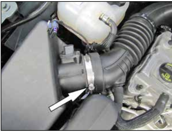
7. Loosen the hose clamp securing the intake tube to the air filter housing.
