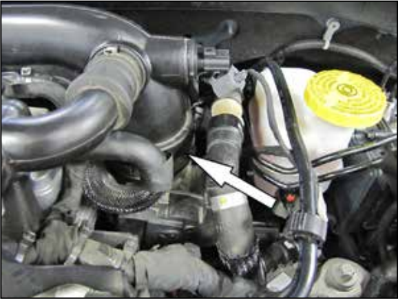
8. Loosen the hose clamp securing the intake tube to the throttle body and then remove the intake tube from the vehicle.
