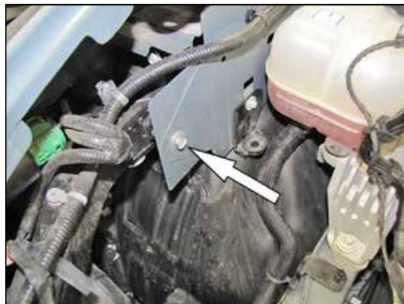
13. Remove the inner fender bolt shown. NOTE: This bolt will be reused in the next step.
