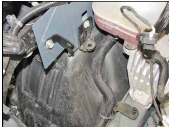
14. Install the heat shield mounting bracket (070712) onto the inner fender and secure with the factory bolt from the previous step.
