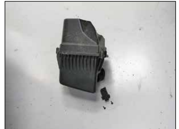
19. If the vehicle is equipped with a humidity sensor, remove the humidity sensor from the factory air filter housing.
