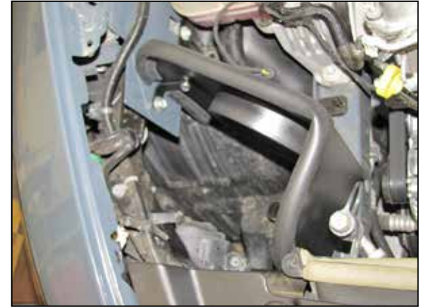
18. Install the heat shield assembly onto the brackets installed previously using the provided hardware.
