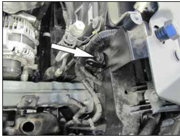
12. Install the provided heat shield mounting bracket (064323) onto the core support and secure with the factory bolt removed in the previous step.
