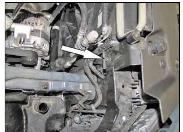
20. On vehicle equipped with a humidity sensor, install the sensor into the K&N® intake tube. On all other vehicles install the provided gasket onto the block off plate and install the block off plate onto the K&N® intake tube.
