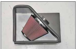
9. Install the K&N® air filter onto the filter adapter and secure with the provided hose clamp. NOTE: Drycharger® air filter wrap; part # RF-1048DK is available to purchase separately.
