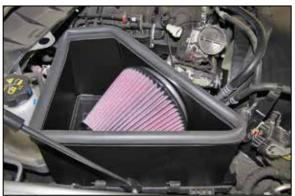
10. Install the heat shield/filter assembly onto the lower air filter housing and secure with the four factory lid retaining clips.
