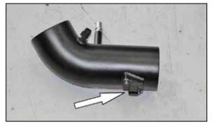
14. Install the humidity sensor into the K&N® intake tube and secure with the provided hardware. NOTE: On vehicles not equipped with a humidity sensor, install the provided block off and gasket.
