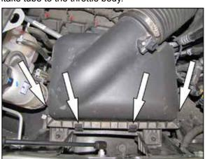
6. Release the four locking tabs securing the air filter housing lid and then remove the housing lid and factory intake tube from the vehicle. Remove the factory air filter.
