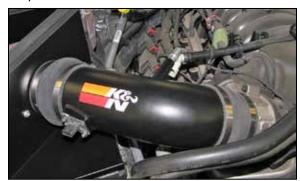
17. Install the K&N® intake tube into the hump coupler and then into the step coupler, then adjust the tube for best fit and secure with the provided hose clamps.
