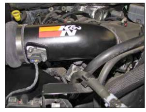
19. Reconnect the humidity sensor and inlet air temperature sensor electrical connections.
