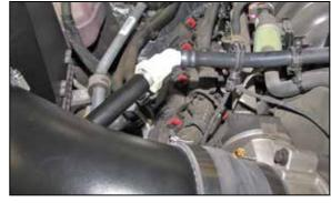
18. Connect the factory crankcase vent hose to the quick disconnect fitting on the K&N® intake tube.
