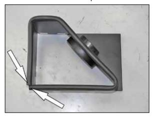
8. Install the provided edge trim onto the K&N $^{\! \otimes \!}$  heat shield as shown.
