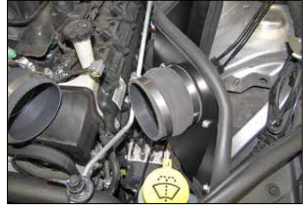
18. Install the provided coupler (08418) onto the filter adapter and secure with the provided hose clamp.
