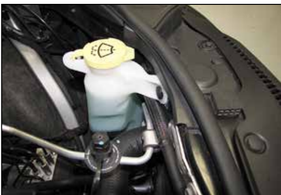
11. Secure the windshield washer bottle to the core support using the factory retaining clip from step #8.
