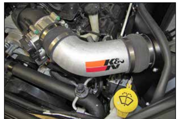
21. Install the K&N® intake tube into the hump coupler and then into the straight coupler, adjust the intake tube for best fit and then secure with the provided hose clamps.
