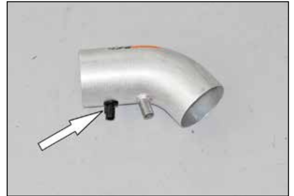
20. Install the provided grommet into the K&N® intake tube. Remove the O-ring from the inlet air temperature sensor and then install the sensor into the grommet as shown.
