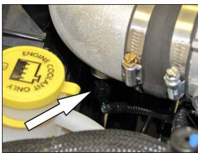
33. Reconnect the inlet air temperature sensor electrical connection and then reinstall the engine cover.
