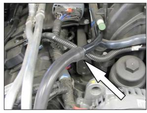
32. Connect the open end of the crank case vent hose to the factory crank case vent tube as shown.
