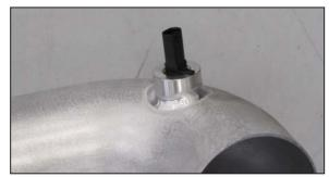
28. Install the inlet air temperature sensor into the K&N® intake tube as shown.
