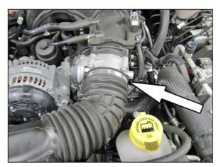
5. Loosen the hose clamp securing the factory intake tube to the throttle body.
