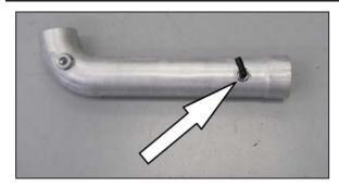
25. Install the 90°,  $\frac{1}{2}$ " vent fitting into the K&N® intake tube as shown.
