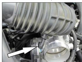
6. Lift up the intake tube and then disconnect the inlet air temperature electrical connection. Then remove the intake tube from the vehicle.
