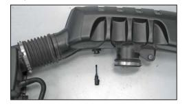
18. Release the locking tab and then remove the inlet air temperature sensor from the factory intake tube by twisting counter clockwise.NOTE: The inlet air temperature sensor is very fragile; take care to avoid damage while
