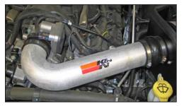
21. Install the K&N<sup>®</sup> intake tube into the hump hose at the filter adapter and then into the hose at the throttle body. Adjust the tube and heat shield for best fit and clearance and then secure with the provided hose clamps rattles and fix as necessary.
