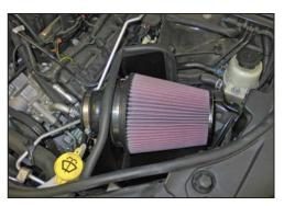
16. Install the K&N<sup>®</sup> air filter onto the adapter and secure with the provided hose clamp. NOTE: Drycharger<sup>®</sup> air filter wrap; part # RF-1041DK is available to purchase separately.
