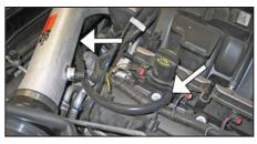
22. Install the crank case vent hose onto the 90° vent fitting and then attach the open end to the valve cover port.
