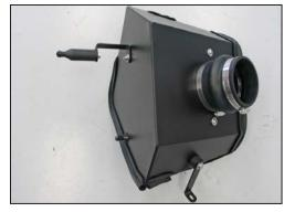
16. Attach the short standoff assembly to the heat shield and secure with the provided hardware as shown.
