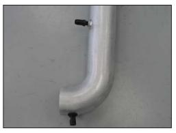
22. Install the inlet air temperature sensor into the grommet previously installed during step #21. NOTE: The inlet air temperature sensor is very fragile, use care when installing the sensor.
