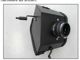
15. Install the bracket/stand-off assembly onto the heat shield using the hardware provided as shown.
