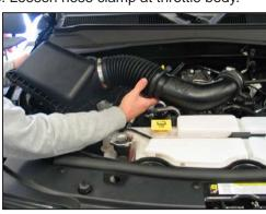
6. Remove the upper airbox and intake tube assembly from the vehicle.
