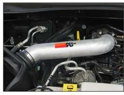
23. Install K&N® intake tube into the silicone hose at the filter adapter and then into the silicone hose on the throttle body. Secure the intake tube with the provided hose clamps.
