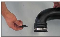
21. Remove inlet air temperature sensor from factory tube as shown.
