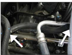
25. Install the crankcase vent hose onto the NPT fitting on the K&N® intake tube. Install the hose mender end into the factory elbow on the valve cover.
