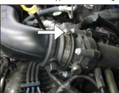
5. Loosen hose clamp at throttle body.
