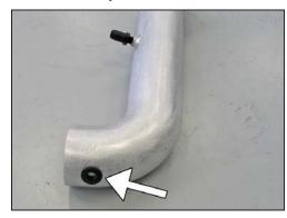
20. Install the provided grommet into the K&N® intake tube as shown.
