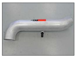
19. Install the provided NPT vent fitting into the  $K\&N^{\tiny\textcircled{\tiny{1}}}$  intake tube as shown.
