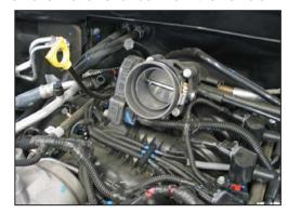
8. Install the silicone hose (084034) onto the throttle body and secure with the provided hose clamp.
