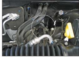
3. Disconnect the crankcase vent hose at the rear of engine, leaving elbow attached to cylinder head.
