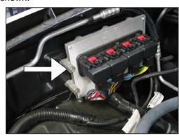
17. Remove the front upper ECU mounting bolt shown.
