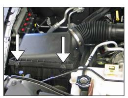
4. Release the two upper airbox retaining clips.
