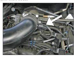
2. Release the red locking tab and then disconnect the inlet air temp sensor electrical connection.
