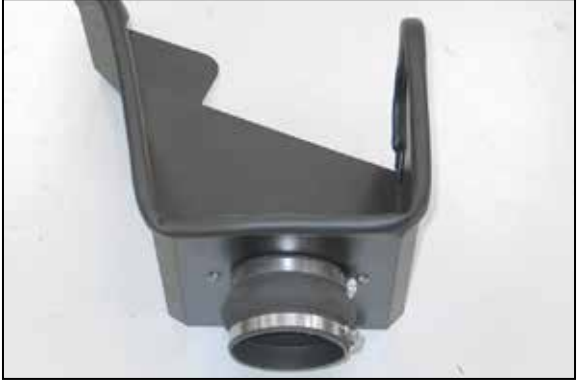
14. Install the silicone hump hose (08418) onto the filter adapter and secure with the provided hose clamp.
