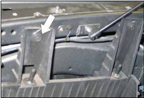
17. Remove the front air box mounting bracket bolt shown. NOTE: This bolt will be used in a later step.
