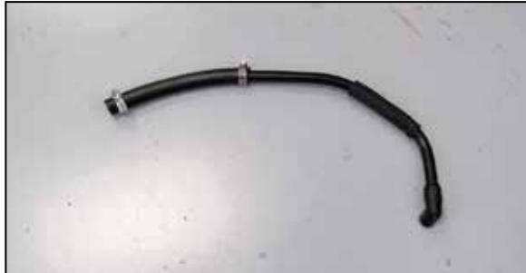
9. Install the provided vent hose onto the cut hose with the provided hose clamps as shown.
