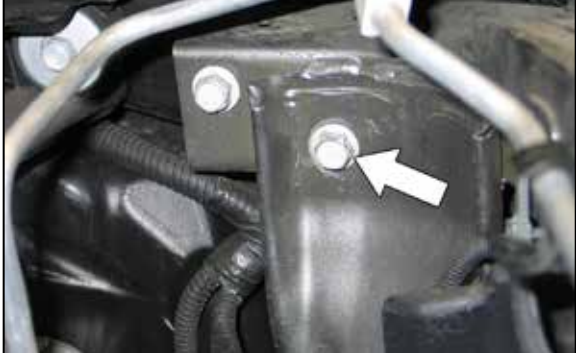
18. Remove the front fender mounting bolt shown. NOTE: This bolt will be used in a later step.
