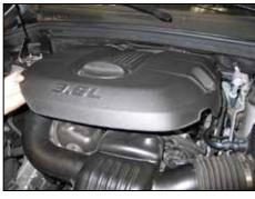
2. Lift up the engine cover to unhook it from the mounting grommets and then remove the engine cover from the engine.
