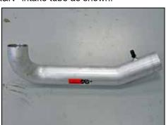
19. Install the provided  $\frac{1}{4}$  npt vent fitting into the K&N® intake tube #27447 as shown.
