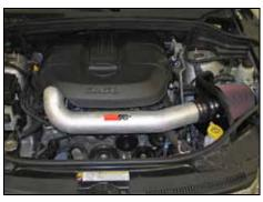
28. Reconnect the vehicle's negative battery cable. Double check to make sure everything is tight and properly positioned before starting the vehicle.
