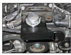
10. Install the provided tube mounting bracket (083150) onto the air injection pump mounting studs, reinstall the air injection pump and secure with the factory mounting nuts from step #9.
