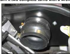
20. Install the provided hump hose (084057) onto to the filter adapter and secure with the provided hose clamp.
