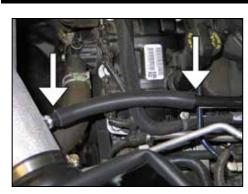
26. Install the provided crank case vent hose onto the vent fitting attached to the K&N® intake tube. Connect the open end of the crank case vent tube to the factory crank case vent tube that was cut in the previous step.
