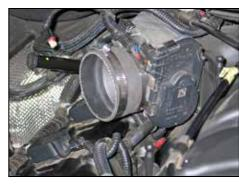
21. Install the provided silicone hose (08690) onto the throttle body and secure with the provided hose clamp.
