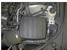
5. Release the two clips that secure the upper air box.
