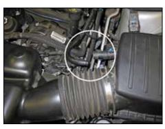
4. Disconnect the crank case vent tube from the air box as shown.
