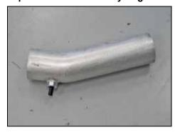
18. Install the inlet air temperature sensor into the  $K\&N^{\circ}$  intake tube as shown.
