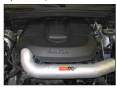
27. Adjust the intake kit for proper fit and then secure the mounting hardware and hose clamps. Reinstall the factory engine cover.
