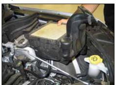
8. Lift up the lower air box to dislodge it from the mounting grommets, then remove the lower air box from the vehicle.
