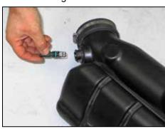
17. Remove the inlet air temperature sensor from the factory intake tube.
