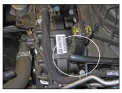
25. Measure the crank case vent tube 5" from the end and then cut off the end with a knife.
