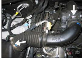
3. Loosen the two hose clamps which secure the stock intake tube to the throttle body and air box, then remove the intake tube from the vehicle.
