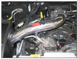
28. Install the K&N® intake tube into the silicone hose at the throttle body and align with the tube mounting bracket installed during step #11. Secure the intake tube with the provided hose clamp and hardware.
