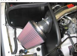
33. Install the filter assembly onto the K&N® intake tube and secure with the provided hose clamp.
