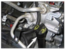
11. Install the tube mounting bracket (010064) onto the A/C compressor and secure with factory bolt removed in the previous step.
