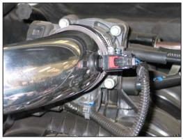
29. Reconnect the inlet air temperature sensor electrical connection.
