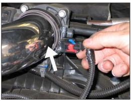
23. On vehicles equipped with and inlet air temperature sensor, install the K&N® intake tube into the silicone hose at the throttle body. Position the inlet air temperature sensor electrical connection for best fit. Mark the location for drilling.
