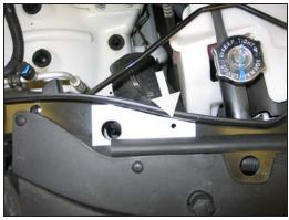
19. Using the provided template, place a mark onto the radiator core support for a hole to be drilled for the heat shield mounting bracket.
