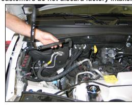
6. Remove the crank case vent tube assembly from the valve cover as shown.
