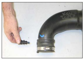
25. Remove the air temperature sensor from the factory intake tube as shown.
