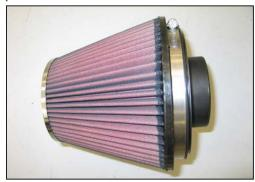
31. Install the filter adapter into the K&N® air filter and secure with the provided hose clamp.
