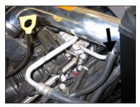
30. Connect the provided silicone vent hose to the modified factory vent tube and then connect the open end to the K&N® intake tube as shown.
