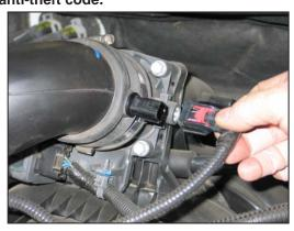
2. Release the red locking tab and then disconnect the temperature sensor electrical connection.
