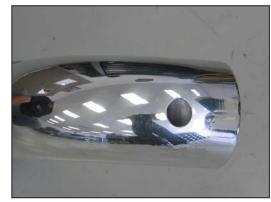
24. Remove the K&N $^{\circ}$  intake tube and drill a  $^{3}$ 4"id hole into the K&N $^{\circ}$  intake tube at the marked location.
