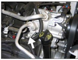
10. Remove the lower rear A/C compressor mounting bolt shown.
