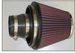
32. Install the provided silicone hose (084055) onto the filter assembly and secure with the provided hose clamp.
