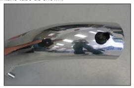
27. Install the air temperature sensor into the grommet installed into the K&N® intake tube as shown.
