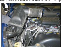
3. Disconnect the stock intake tube from the intake plenum. Then lift to remove to remove the airbox assembly from the vehicle as shown.
