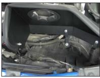
13. Install the heat shield assembly and secure with the provided hardware and the factory mounting nut. Be sure to remove the factory spacer on the airbox mounting stud before installing the heat shield.
