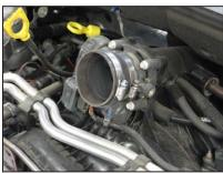
16. Install the provided silicone hose (084036) onto the throttle body and secure with the provided hose clamps.
