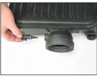
18. Twist the air temperature sensor counter clockwise and remove it from the stock intake plenum.
