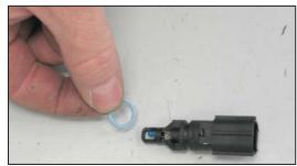
19. Remove the "O" ring from the air temperature sensor.
