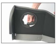
8. Install the provided edge trim onto the heat shield as shown.
