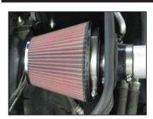
26. Install the air filter assembly onto the K&N<sup>®</sup> intake tube and secure with the provided hose clamp.
