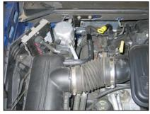
2. Loosen the hose clamp at the throttle body and the airbox mounting nut. Then disconnect the crankcase vent from the inline fitting.
