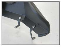
11. Install the "C" bracket (010118) onto the heat shield with the provided hardware as shown.
