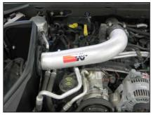
21. Install the K&N® intake tube into the into the silicone hose on the throttle body and position so the tube aligns with the mounting bracket. Secure the tube with the provided hose clamp and hardware.
