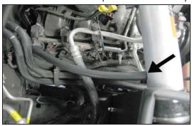
30. Install the provided silicone crankcase vent hose onto the fitting on the engine and then connect to the fitting on the K&N<sup>®</sup> intake tube. **NOTE: Some trimming of the hose may be necessary.**
