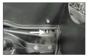
24. Secure the lower heat shield mounting bracket to the stud on the inner fender with the hardware provided.
