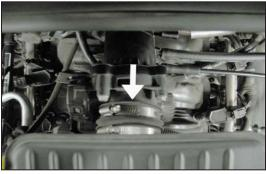
5. Loosen the hose clamp that secures the intake plenum to the throttle body.
