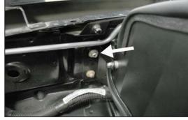
23. On 2007 model year vehicles, secure the upper heat shield mounting bracket with the nut removed in step #11.
