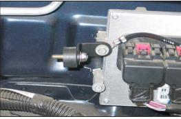
21b. On 2008 and later vehicles, attach the "L" bracket assembly from step #21a. to the ECU using the factory bolt removed in step #11a.
