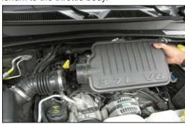
$\label{eq:continuous} \textbf{6. Remove the intake plenum from the vehicle}.$
