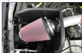
29. Install the filter assembly onto the K&N<sup>®</sup> intake tube and secure with the provided hose clamp.
