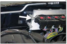
11a. On 2008 and later vehicles, remove the front-upper ECU mounting bolt shown.
