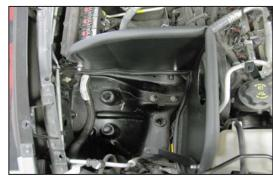
22. Install the heat shield assembly into the vehicle so that the two small "L" brackets align with the threaded stud on the inner fender and the ECU mounting stud.
