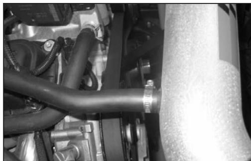
20. Connect the crankcase vent hose to the K&N® intake tube and secure with the provided hose clamp as shown.
