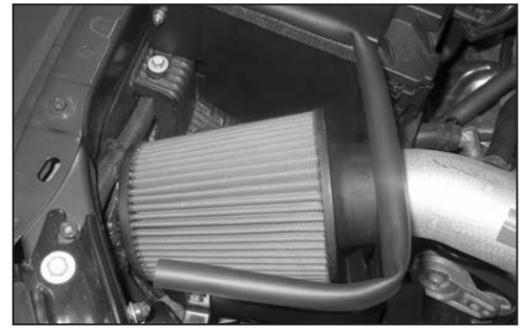
21. Install the K&N® air filter and secure with the provided hose clamp.
