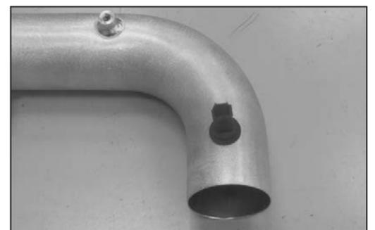
8. Install the air temperature sensor into the grommet installed into the K&N intake tube during step #6.
