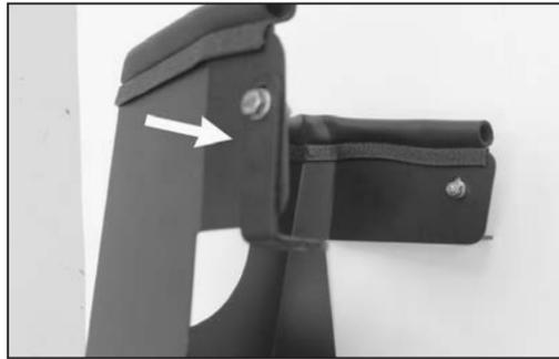
17. Install the supplied "L" bracket (07195) onto the heat shield as shown with the provided hardware.
