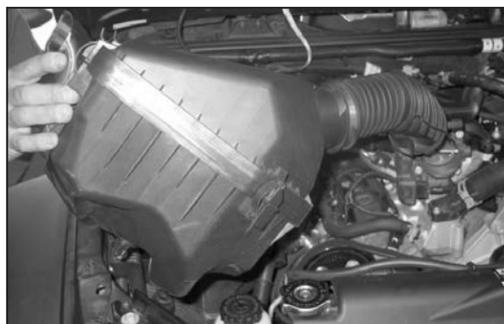
5. Lift up the airbox assembly to dislodge it from the mounting grommets and remove the complete assembly from the vehicle.
