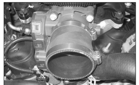
9. Install the supplied silicone hose (08096) onto the throttle body and secure with the supplied hose clamp.
