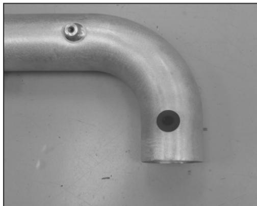
6. Install the supplied grommet into the hole in the K&N intake tube as shown.
