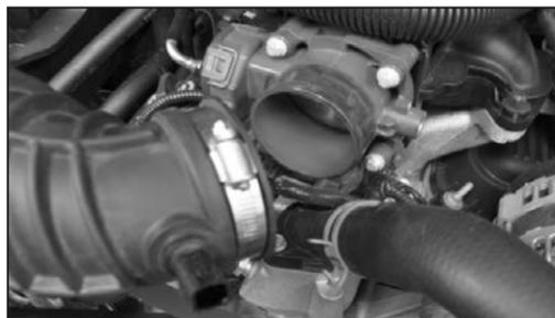
4. Loosen the hose clamp that secures the stock intake tube to the throttle body and then disconnect the intake tube from the throttle body.
