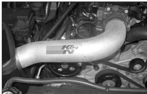
19. Insert the K&N® intake tube into the silicone hose at the throttle body and align with the mounting bracket installed in step #11 and then secure with the hose clamp and hardware provided.
