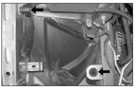
20. Remove the coolant reservoir-retaining nut and air box mounting grommet shown.
