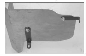
17. Install the short "L" bracket (07158) onto the heat shield as shown with the provided hardware.
