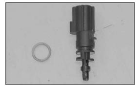
27. Remove the rubber sealing "O" ring from the air temperature sensor as shown.
