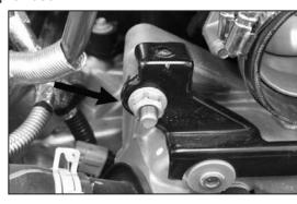
23. Remove the intake plenum mount nut shown. **NOTE: Do not discard as this nut will be reused.**
