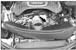
5. Pull the intake plenum off of the throttle body and rotate forward, then disconnect the crank case vent hose from the tube attached to the intake plenum.
