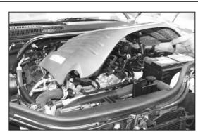
7. Remove the engine cover from the engine.
