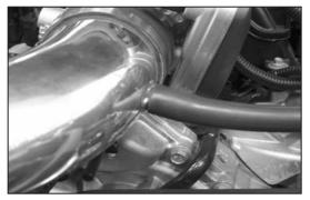
30. Install the provided crank case vent tube onto the valve cover and then onto the K&N<sup>®</sup> intake tube as shown.
