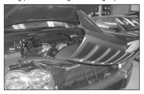
11. Remove the six grill retaining clips from the grill, then tilt the grill forward and lift to remove from the vehicle.
