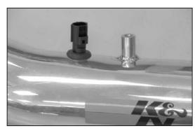
28. Install the air temperature sensor into the grommet installed into the K&N® ntake tube in step #25.
