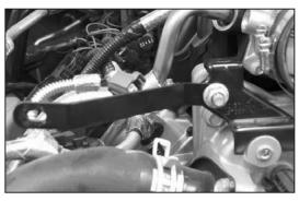
24. Install the tube mounting bracket onto the plenum mount and secure with the factory nut removed in step #23.
