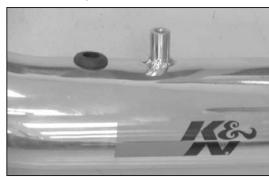
25. Install the provided grommet into the  $K\&N^{\otimes}$  intake tube as shown.
