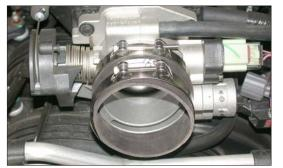
16. Install the provided silicone hose (084031) onto the throttle body and secure with the provided hose clamp as shown.
