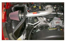
27. Reconnect the vehicle's negative battery cable. Double check to make sure everything is tight and properly positioned before starting the vehicle. 28. The C.A.R.B. exemption sticker, (attached), must be visible under the hood so that an emissions inspector can see it when the vehicle is required to be tested for emissions. California requires testing every two years, other states may vary.
