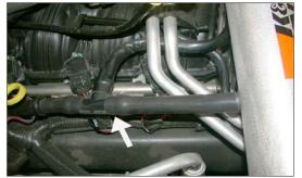
23. Install the provided crank case vent hose onto the factory "TEE" fitting and then onto the K&N<sup>®</sup> intake tube as shown.
