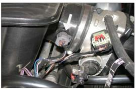
4. Depress the locking tab on the air temperature sensor electrical connection and then pull to disconnect the sensor electrical connection.
