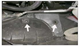
6. Pull the two-air box mounting grommets shown from the inner fender.
