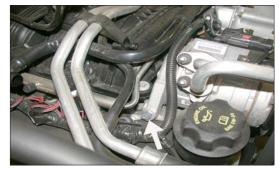
14. Remove the rear, lower A/C compressor mounting bolt shown.
