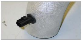
20. Install the sensor into the grommet installed in step #18.
