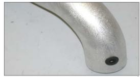
18. Install the provided grommet into the  $K\&N^{\ensuremath{\mathbb{R}}}$  intake tube as shown.
