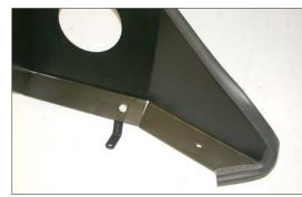
9. Install the "Z" bracket (010120) onto the heat shield with the provided hardware as shown.
