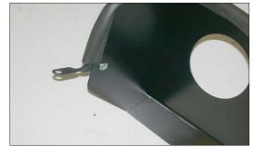
8. Install the twist bracket (070702) onto the heat shield with the provided hardware as shown.
