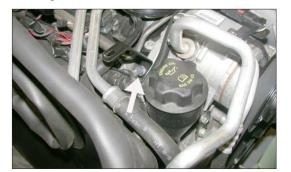
15. Install the tube mounting bracket (010119) onto the A/C compressor using the bolt removed in step #14 as shown.
