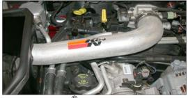
21. Install the K&N<sup>®</sup> intake tube into the throttle body hose and position so the mounting bracket aligns with the tube mounting stand off and then secure with the provided hardware.
