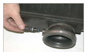
17. Twist the air temperature sensor counter clockwise and remove it from the stock intake
