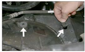
12. Install the two threaded inserts into the air box mounting grommet locations as shown.
