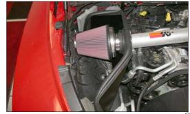
26. Install the air filter assembly onto the K&N<sup>®</sup> intake tube and secure with the provided hose clamp as shown.
