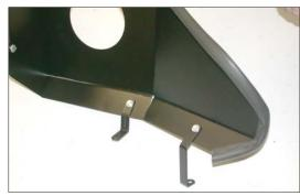
10. Install the "C" bracket (010118) onto the heat shield with the provided hardware as shown.
