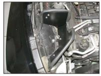
14. Install the heat shield assembly and secure with the provided hardware and the factory airbox mounting nut.
