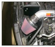
26. Install the air filter assembly onto the K&N<sup>®</sup> intake tube and secure with the provided hose clamp as shown.
