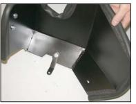
10. Install the "L" bracket (010122) onto the heat shield with the provided hardware as shown.
