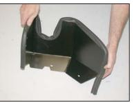
8. Install the provided edge trim onto the heat shield as shown.
