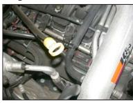
23. Install the provided crankcase vent hose onto the factory crankcase vent fitting and then onto the  $K\&N^{\mbox{\tiny (B)}}$  intake tube as shown.
