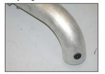
17. Install the provided grommet into the  $K\&N^{\otimes}$  intake tube as shown.
