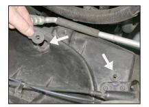
13. Install the two threaded inserts into the airbox mounting grommet locations as shown.
