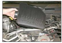
6.Lift and remove the intake plenum from the vehicle as shown.
