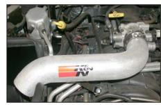
21. Install the K&N<sup>®</sup> intake tube into the silicone hose at the throttle body and position so that the mounting bracket aligns with the plenum mounting location. Then secure with the provided hardware.
