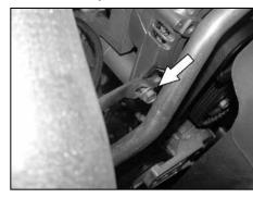
22. Rotate the bracket onto the hex bolt from step 10 and snug the bolt, but do not completely tighten at this time.
