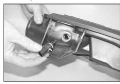
17. Twist the temp sensor counter clockwise to unlock and remove the temp sensor from the resonator.
