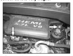
8. Remove the two 10mm resonator retaining bolts, then remove the resonator from the vehicle.
