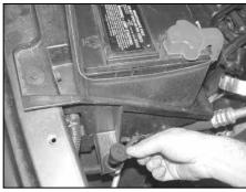
14. Install the 3/8" threaded insert provided into the air box mounting grommet hole vacated in step #14.
