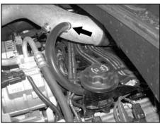
24. Connect the provided silicone hose to the crank case vent on the oil fill tube, then, connect the other end to the vent on the intake tube as shown.
