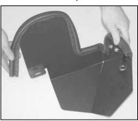
12. Install the provided edge trim onto the heat shield. Trim if necessary.
