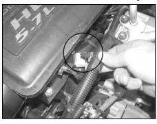
6. Unclip the engine wire harness clip from the resonator box as shown.
