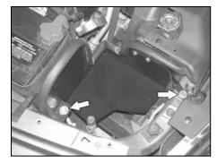
15. Install the heat shield assembly and secure the mounting bracket to the radiator core support with original bolt removed in step #13. Secure the rear of the heat shield to the 3/8" threaded insert with the provided hardware.
