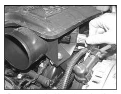
7. Depress the locking tab on the air temp sensor and disconnect its electrical connection.
