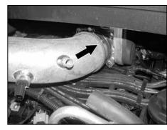
21. Slide the intake tube into the silicone hose on the throttle body as shown.
