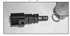
18. Remove the O-ring from the air temp sensor as shown.
