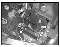
13. Remove the core support mounting bolt shown with a 13mm wrench, and pull out the stock air box mounting grommet shown.
