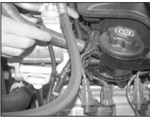
2. Disconnect the crank case vent hose at the oil filler stand off as shown.
