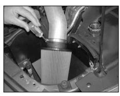
26. Install the K&N® air filter and secure with the provided hose clamp as shown.
