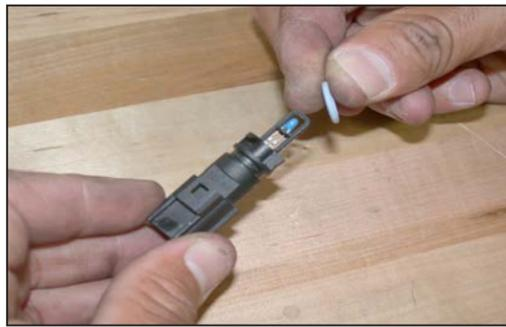
21. Remove the o-ring from the stock air temperature sensor as shown.
