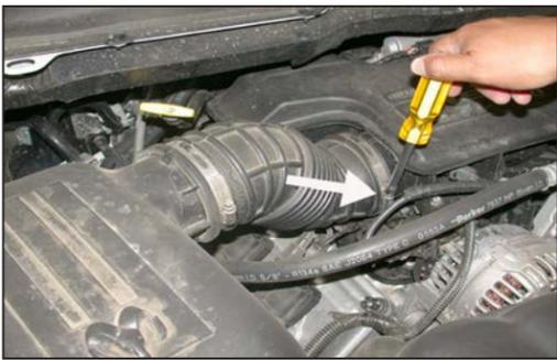
2. Loosen the hose clamp at the intake resonator as shown.
