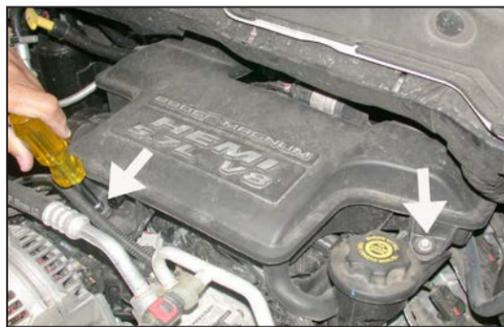
5. Loosen the two bolts that secure the intake resonator to the manifold as shown.
