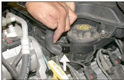
6. Disconnect the crankcase vent hose as shown.
