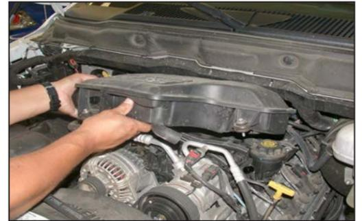
7. Pull firmly upwards to remove the air intake resonator as shown.
