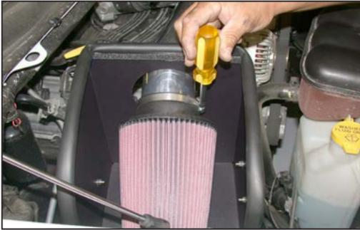
30. Install the K&N® air filter onto the intake tube and secure with the provided hose clamp as shown.
