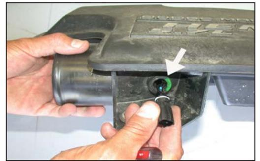
8. Turn the air temperature sensor 1/4 turn, then, remove the air temperature sensor from the air intake resonator as shown.
