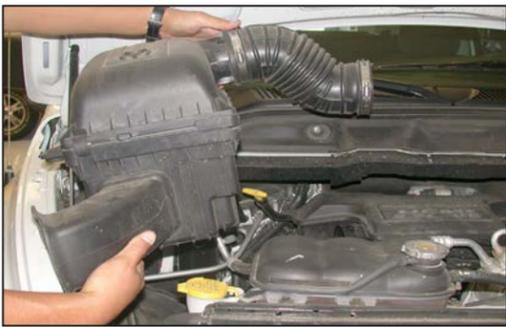
3. Disconnect the intake tube, then, pull firmly upwards to remove the air cleaner assembly as shown.
