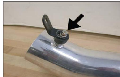
23. Install the angled bracket onto the rubber mounted stud using the provided hardware as shown, but do not tighten completely at this time.
