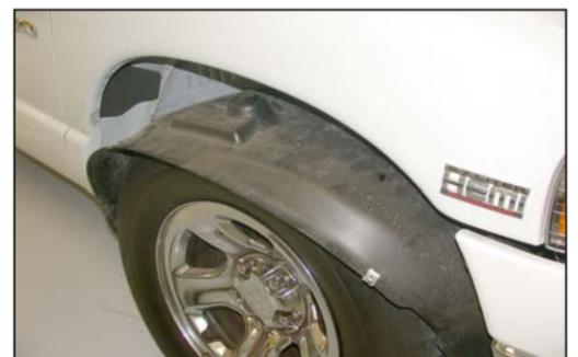
9. Loosen and remove the 8 bolts that secure the inner fender valance, then, lower the valance down as shown.
