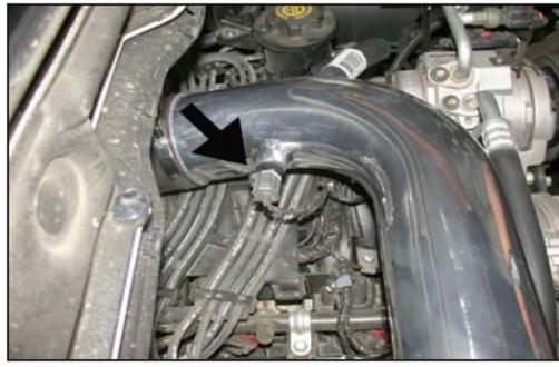
31. Reconnect the air temperature sensor electrical connection as shown.
