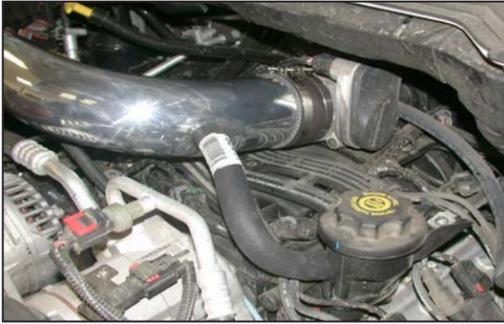
29. Attach the provided 5/8" id crank case vent hose onto the appropriate fitting on the K&N® intake tube, trim for proper fitment to prevent the hose from developing a kink and attach the open end to the crank case vent port.
