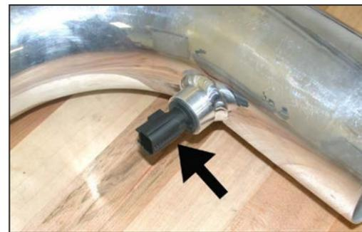
25. Slide the air temperature sensor into the silicone hose as shown.
