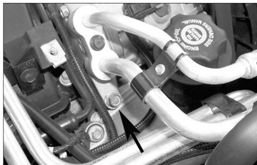
18. Remove the bolt from the A/C compressor as shown.
