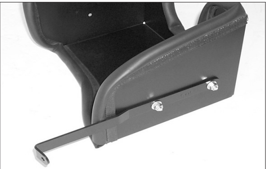
11. Install the provided large "L" bracket onto the heat shield as shown. Do not tighten completely.
