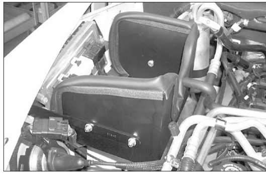
14. Install the heat shield into the vehicle as shown.
