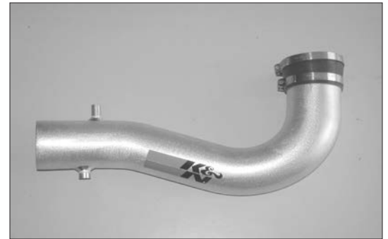
20. Install the silicone hose onto the K&N® intake tube as shown.
