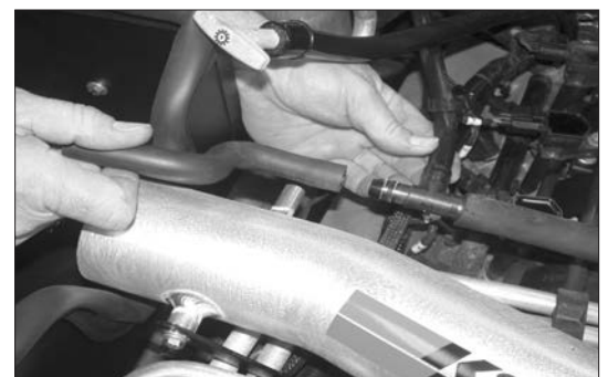
22. Remove the vent hose from vehicle as shown.
