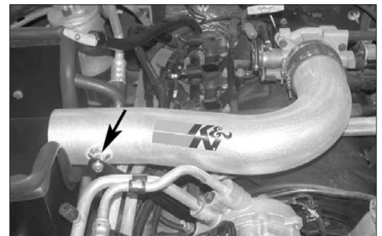
21. Install the K&N® intake tube onto the throttle body and secure with the provided hose clamp, then secure to the tube mounting bracket installed in step #19 with the provided hardware as shown.
