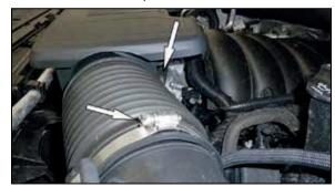
4. Loosen the hose clamps that secures the intake plenum to the air filter housing and to the throttle body. Disconnect the plenum connections at the air filter housing and then rotate the plenum counter clockwise to disengage the keyed mount and separate it from the throttle body.
