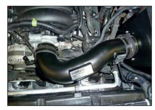
22. Install the intake tube into the coupler at the filter adapter and then into the coupler at the throttle body, adjust the tube for best fit and then secure with the provided hose clamps.
