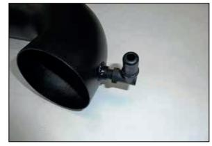
20. Install the provided  $90^{\circ}$  quick connect fitting into the K&N® intake tube as shown.
