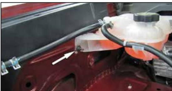
11. Remove the nut that secures the coolant reservoir to the inner fender.
