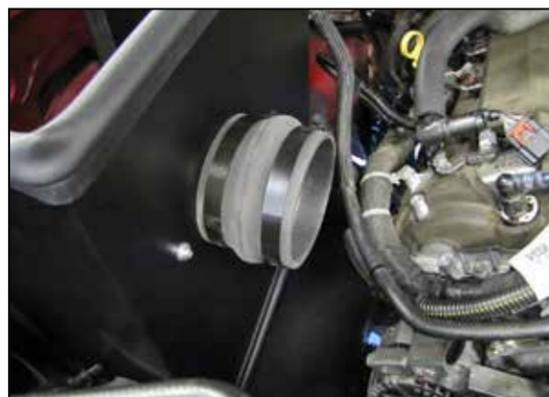
18. Install the intake tube assembly into the coupler at the filter adapter and then into the coupler on the throttle body. Adjust the tube for best fit and secure with the provided hose clamps.
