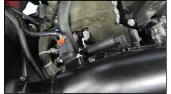
20. Using the provided vent hose, connect the factory vent to the 90° fitting installed into the K&N® intake tube. Reconnect the mass air sensor electrical connection.
