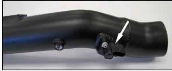
13. Remove the mass air sensor from the factory air filter housing and install the sensor into the K&N® intake tube using the provided hardware.
