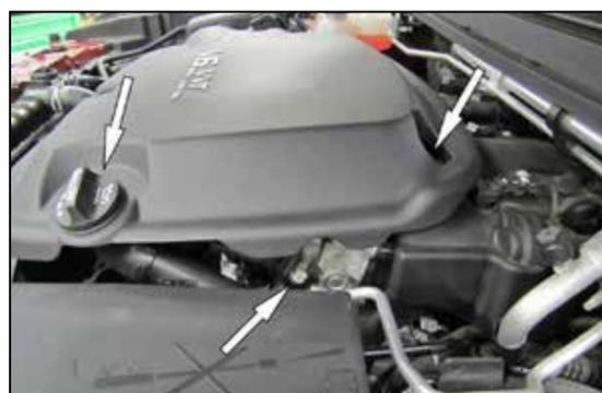
3. Remove the oil fill cap and loosen the hose clamp securing the intake hose to the throttle body. Remove the bolt securing the intake plenum to the engine.
