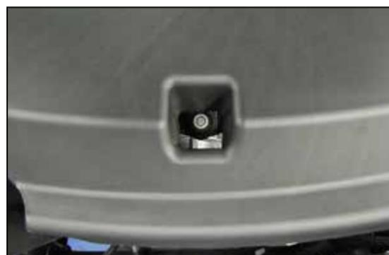
4. Remove the front center bolt securing the intake plenum to the engine and remove the plenum from the vehicle.
