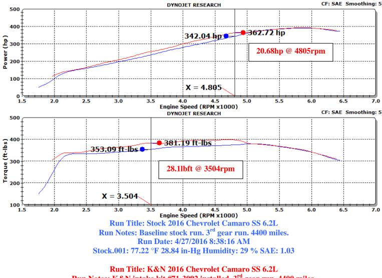
Run Notes: K&N intake kit #71-3092 installed. 3<sup>rd</sup> gear run. 4400 miles. Run Date: 4/27/2016 10:16:37 AM K&N.002: 85.61 °F 28.88 in-Hg Humidity: 20 % SAE: 1.03
