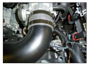
12. Install the intake tube into the coupler at the filter adapter and then into the coupler at the throttle body, adjust the tube for best fit and then secure with the provided hose clamps.
