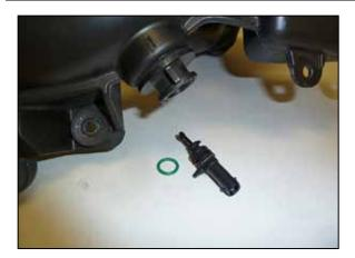
7. Remove the temp sensor from the factory intake tube by gently lifting the tab and rotating the sensor counter clockwise. Once the sensor is removed, remove the sealing O ring from the sensor. **NOTE: The temp sensor is very fragile, use care while handling.**
