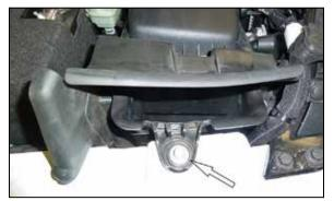
4. Remove the bolt shown that secures the fresh air intake duct to the fender, then lift and remove the complete intake system from the vehicle. NOTE: The factory mounting grommets should remain in the vehicle. NOTE: K&N Engineering, Inc., recommends that customers do not discard factory air intake.
